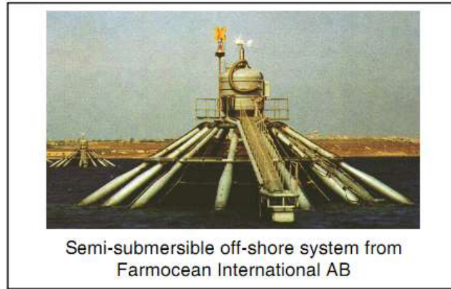
Gambar 2.2 Aquaculture semi-submersible offshore system (Fermocean) (Scott D.C.B.,Munir J.F, 2000)
