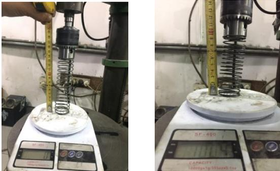
Gambar 4. 1 Mencari konstanta pegas *shaker* TST
