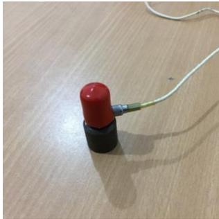
Gambar 4. 14 Probe Accelerometer
