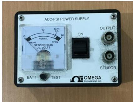
Gambar 4. 15 Power Supply Accelerometer
