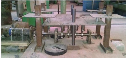
Gambar 2. 5 Alat Vibration Exciter cam and follower
