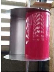
**Gambar 3.4** Turbin Angin Savonius
