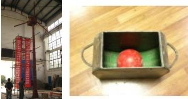
Gambar 2. 5 (a) Model turbin angin dan (b) *Ball Vibration Absorber* [5]
