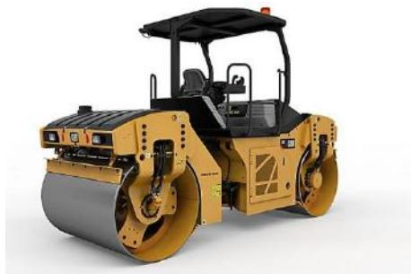
**Gambar 5.20 Alat Tandem Roller**
