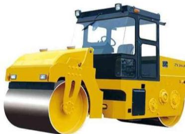
**Gambar 5.17 Alat Vibro Roller**
