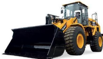
**Gambar 5.16 Alat Wheel Loader**
