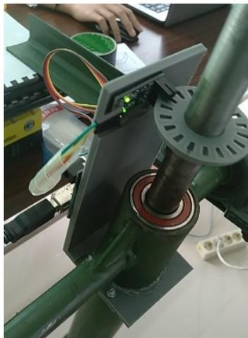
Gambar 3.5 *Sensor Rotary Encoder*
