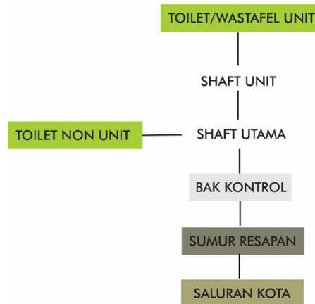
Gambar 4.2.2 - Diagram alur air kotor
