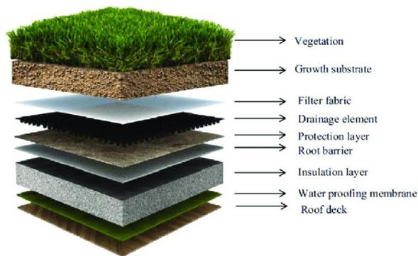
Gambar 4. 6 Sistem Lapisan *Green Roof*
