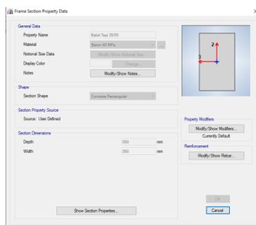
Gambar 4 19 Input Section Properties
