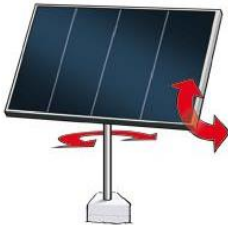
Gambar 2. 3 Dual Axis Solar Tracker [12]
