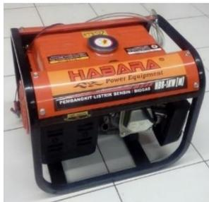
**Gambar 2.2** Generator set biogas
