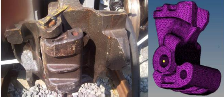
Gambar 2.4 Forged coupler knuckle and mesh (Wang et al., 2013)
