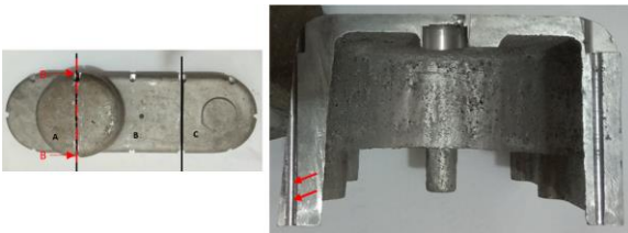
Gambar 4.18 Cacat shrinkage porosity cover CVT bagian B potongan B-B
