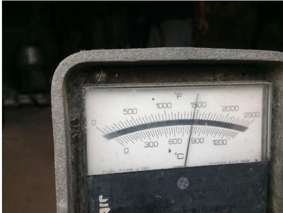
Gambar 3.7 Temperatur tuang aluminium paduan Al-Si
