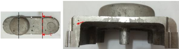
Gambar 4.19 Cacat gas porosity cover CVT bagian B potongan C-C
