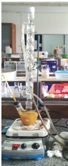
Gambar 4.5 Rangkaian refluks sintesis biodiesel
