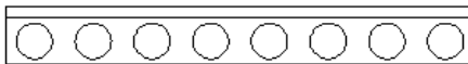
Gambar 2.7 Hollow Core Slab ( PCI Design Handbook 7 th Edition Precast and Prestressed Concrete, 2010 )
