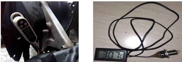
*Gambar 3.2 Thermometer Digital*
