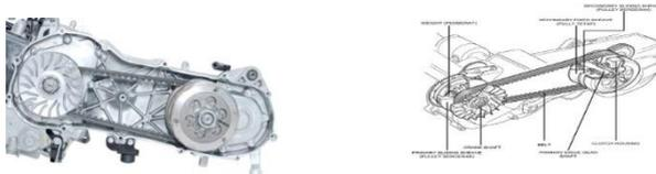
Gambar 2.7 Drive Pulley [6]
