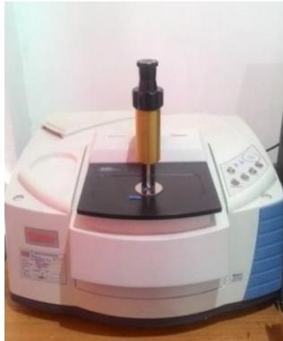
**Gambar 3.1** FTIR (*Fourier Transform Infrared*)
