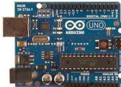
Gambar 4.4 Papan Arduino Uno
