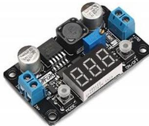
Gambar 4.7 Modul step down LM2596
