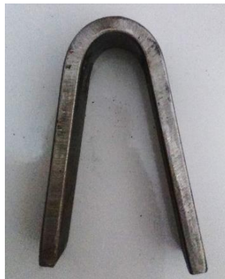
Gambar 4.13. Hasil Uji Root Bend Pengelasan Gap 2 mm tanpa Backing Ceramic
