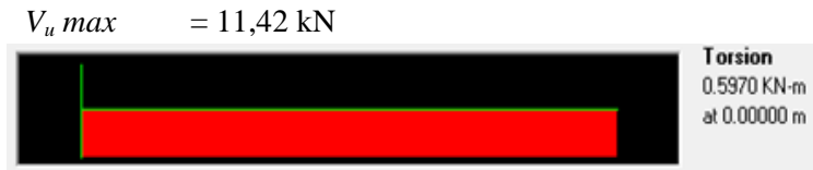
Gambar 7. 21 Diagram Torsi Balok Kantilever
