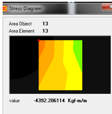
Gambar 7. 5 Diagram Momen M11 Dinding Basement
