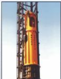
SGH-3013 30ton RAM WEIGHT with 1.3m STROKE
