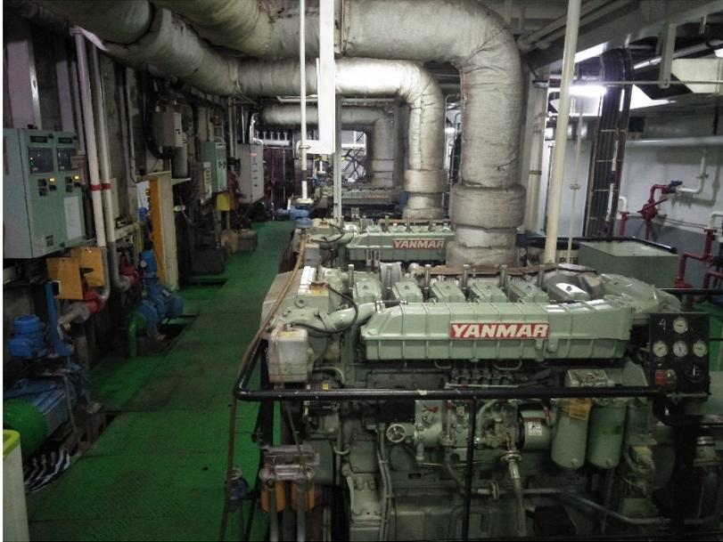
*Gambar 4. 3 auxiliary engine YANMAR*
