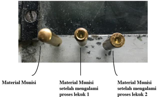
**Gambar 4.5** Gambaran Proses Mesin Lekuk 3DD
