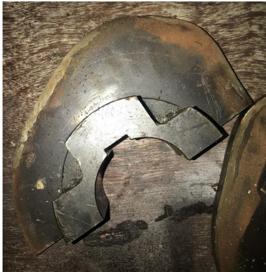
**Gambar 4.2** Komponen Cam Sistem Penahan Kerja Aus
