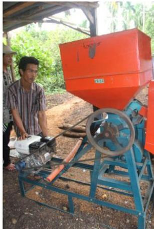
**Gambar 3.5** Pengupasan Kulit Tanduk (Hulling)
