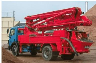
Gambar 2. 7 Concrete Pump
