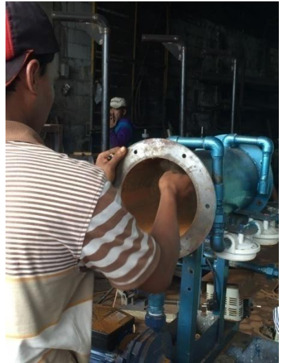
Figure 1. 4 Rust removal from UV reactor.
