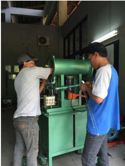
Figure 1. 1 Installing the UV glass protector
