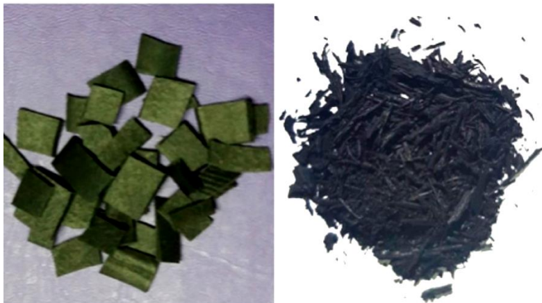
Figure 10 Crumb rubber from the previous experiment (left), crumb rubber used in this experiment (right)
