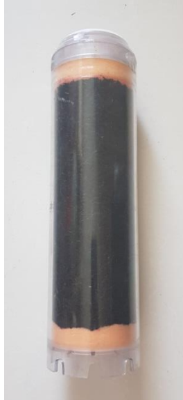
Figure 23 Sponge (orange color) on the top and bottom side of crumb rubber.
