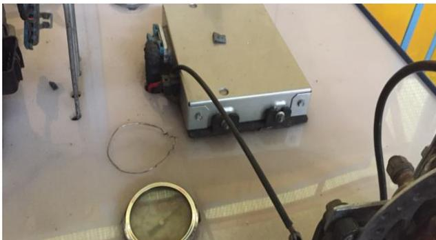
**Gambar 2. 5** *Electronic Control Unit*
