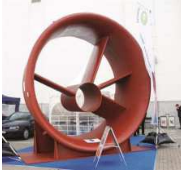
Gambar 2. 16 Marvis Duct ( Sumber : www.wartsila.com )
