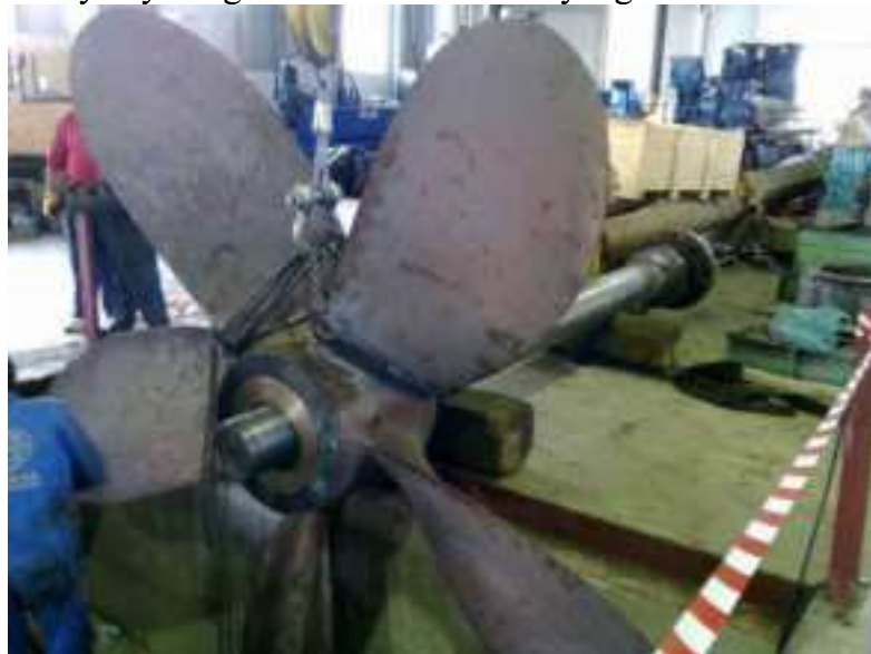
Gambar 2. 10 Keyless Propeller Fabrication ( sources : www.mpss.gr )
