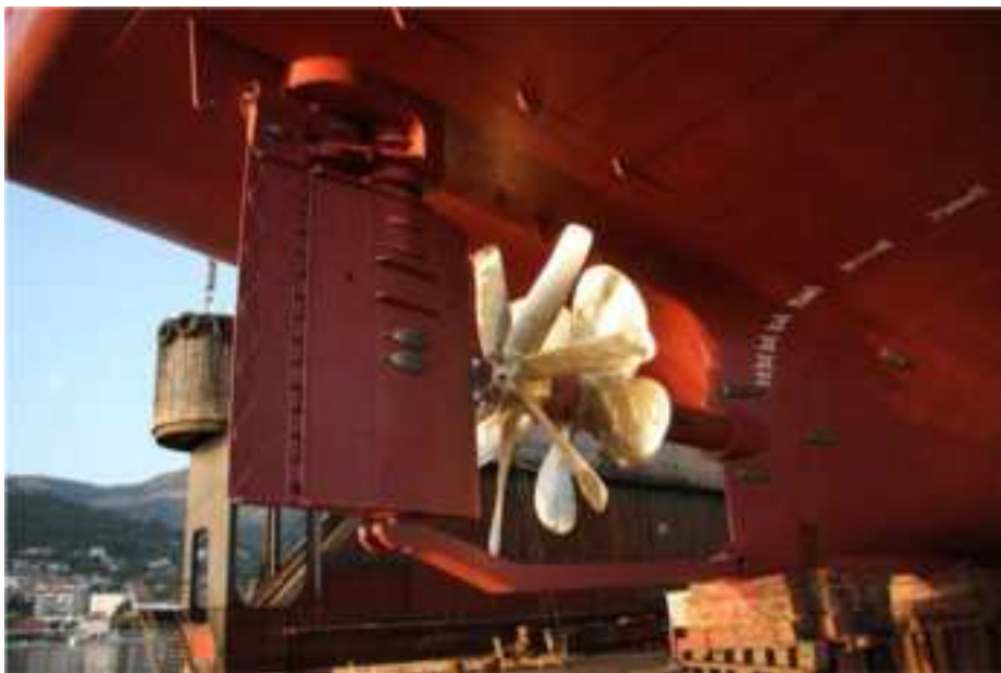
Gambar 2. 18 Grim Vane Wheel ( Sumber : www.upload.wikipedia.org )
