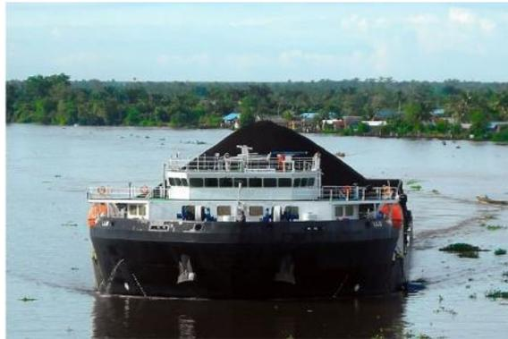
Gambar 2.4 Self Propelled Barge
