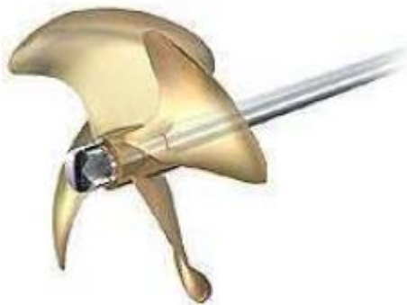
Gambar 2.1 : Fixed Pitch Propeller (Sumber : Sasono J, 2009)
