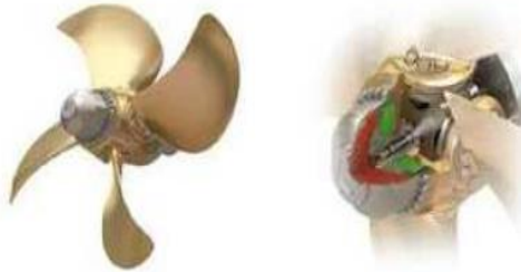
Gambar 2.2 : Controllable Pitch Propeller (Sumber : Sasono J,2009)
