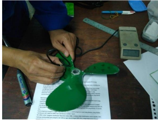
Gambar 3.4 Pengukuran ketebalan coating
