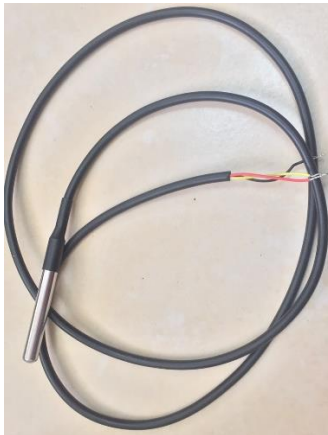
Gambar 2.5 Modul Sensor DS18B20
