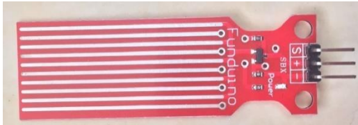
Gambar 2.4 Modul Sensor EK1195
