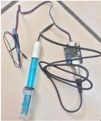
Gambar 2.2 Modul Sensor SEN0161
