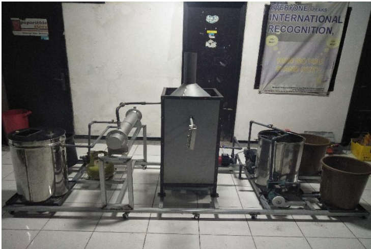
Gambar 4.1 Desalintaion water plant
