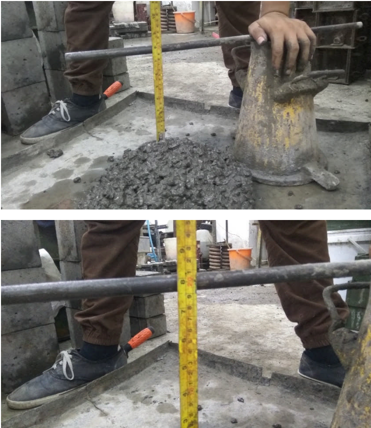
Gambar 4.13 Pengujian Slump Beton Geopolimer 12M Air Suling
