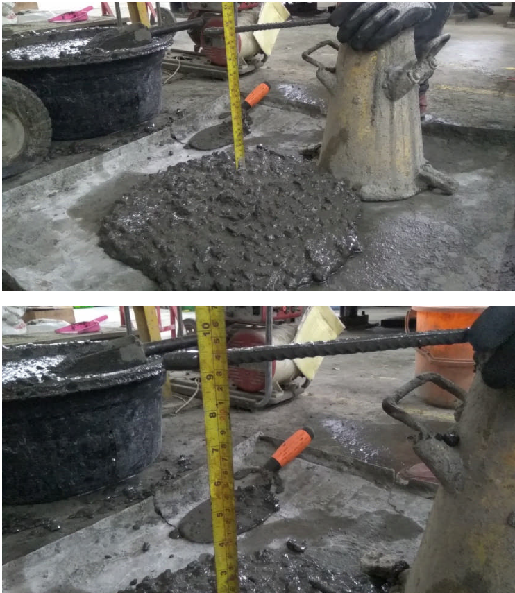
Gambar 4.15 Pengujian Slump Beton Geopolimer 10M Air Suling
