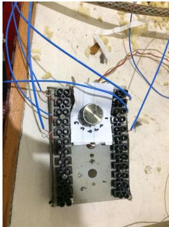
**Gambar 3. 26 *Thermocouple selector***
