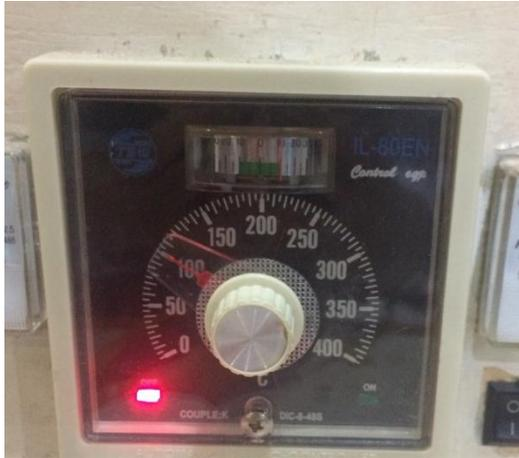
**Gambar 3. 23 Set point adjustment thermocontrol**
