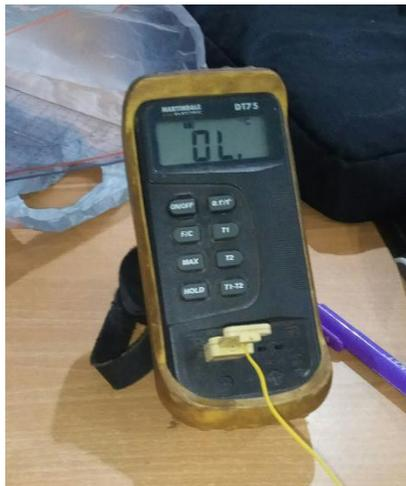
**Gambar 3. 24 Digital thermometer**
