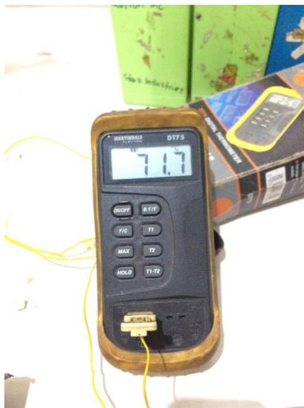
**Gambar 3. 18 Digital Thermometer**
