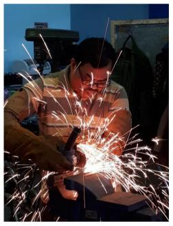
Figure 4. 6 Polishing Specimen Using Grinder
