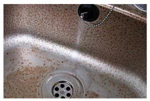
Figure 2. 8 Pitting Corrosion on Sink (Consultants, n.d.)
