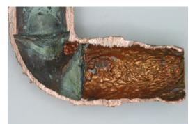
Figure 2. 9 Corrosion Erosion on Seawater Pipe (Bloging, n.d.)
