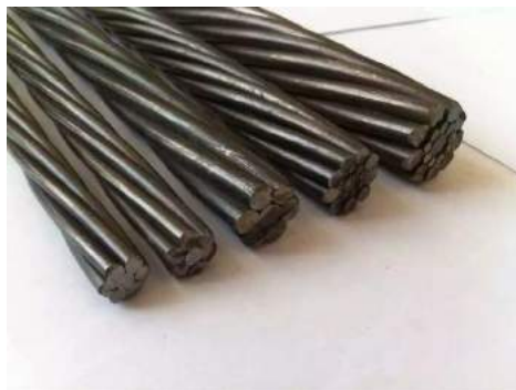
Gambar 2. 8 Baja Prategang ( Prestressing Steel )
