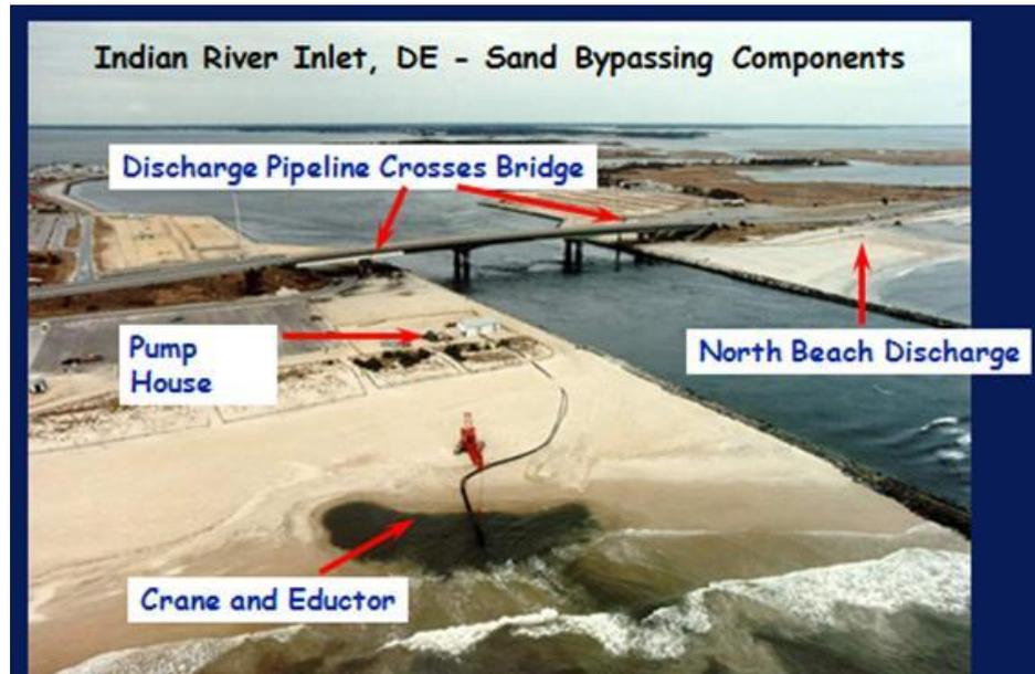
**Gambar 1.4** contoh sand bypassing land based mobile system (sumber : Boswood, 2001)
