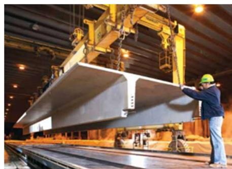
*Gambar 10 Doble-tee Slab
