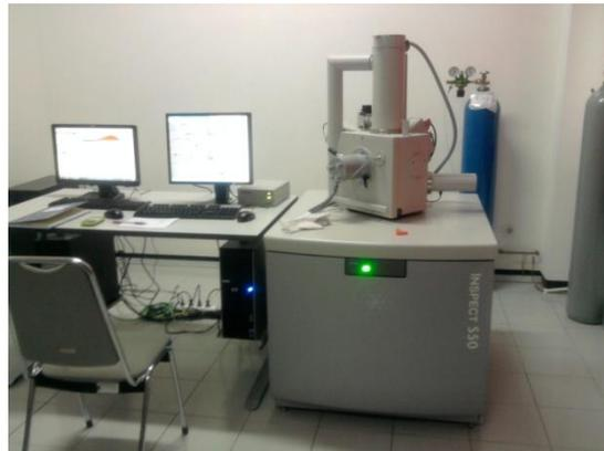
Gambar 3. 4. Scanning Electron Microscope (SEM) S50
