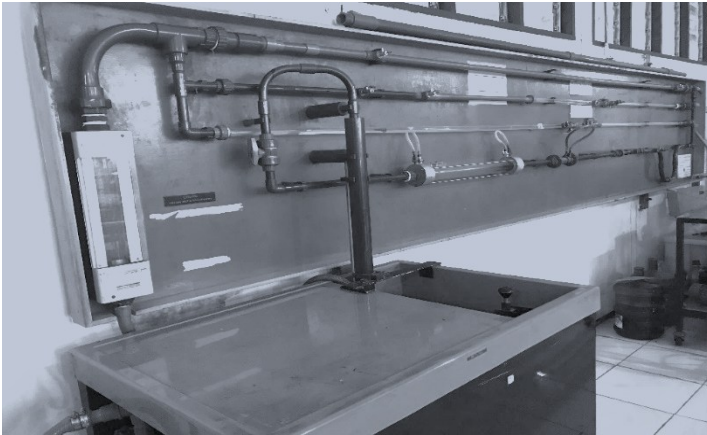
Gambar 3.2 Instalasi alat uji CUSSONS friction loss in pipe apparatus
