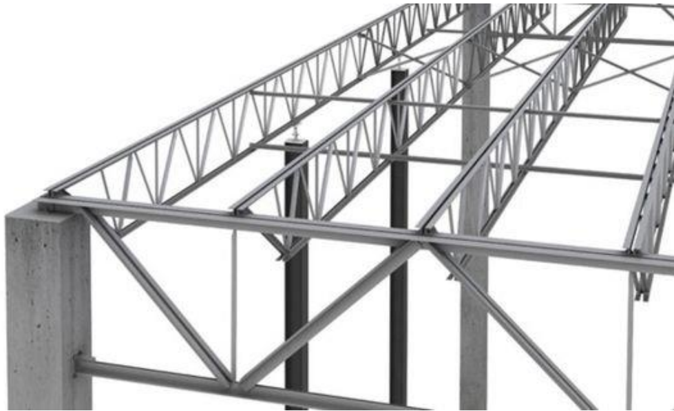
Gambar 4.11 Rangka Atap Flat Truss Standart
