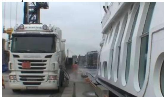
**Gambar 2.6. LNG Truck to Ship Bunkering**
