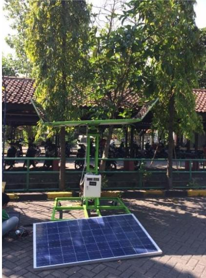
**Gambar 3. 6** Prototipe active solar tracker
