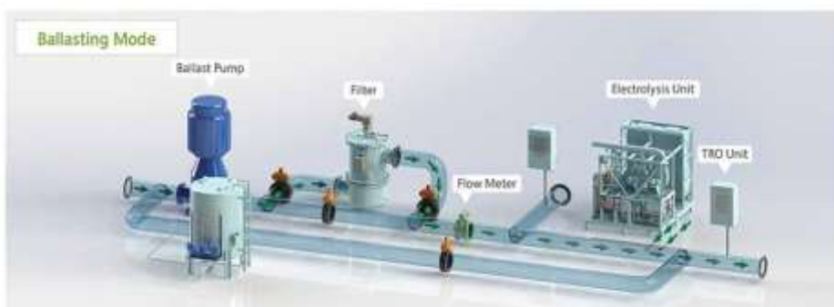
Figure 2. 5Ballasting mode of electrolysis ballast water treatment (Source: Purimar)
