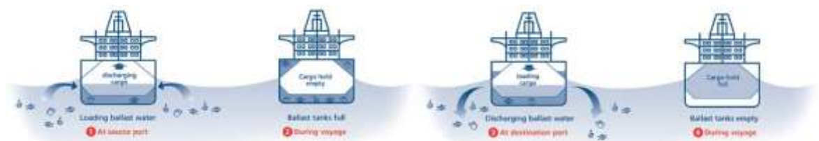
Figure 2. 3Process of take in and discharge of ballast water that contain organic matter (Source: IMO)
