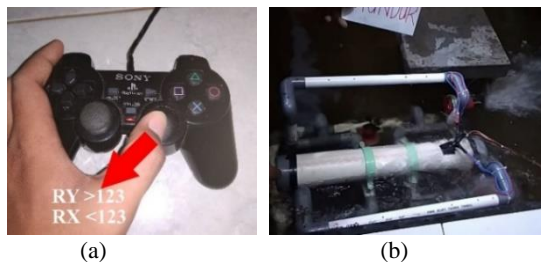
Gambar 4.13 (a) Perintah Joystick Mundur (b) Gerakkan ROV Mundur
