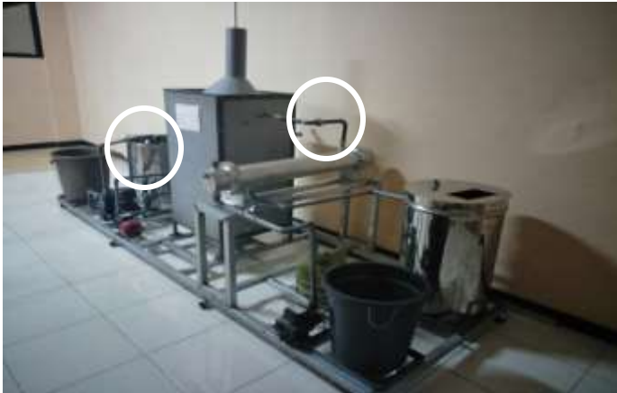
Gambar 4.1 Mini Desalination Water Plant
