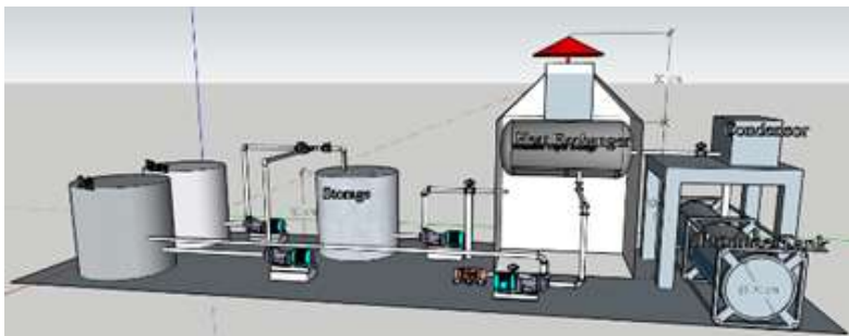
Gambar 3.4 Desain 3D Mini Desalination Water Plant
