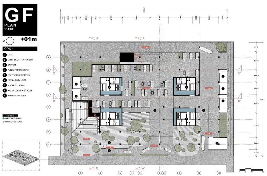
Gambar 5.5. ground floor plan
