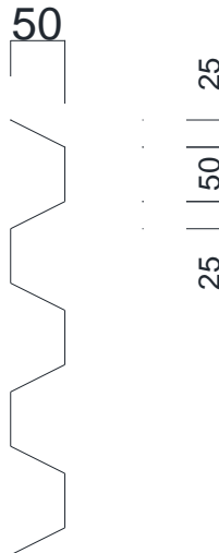
Gambar 4. 52 desain Shear key
