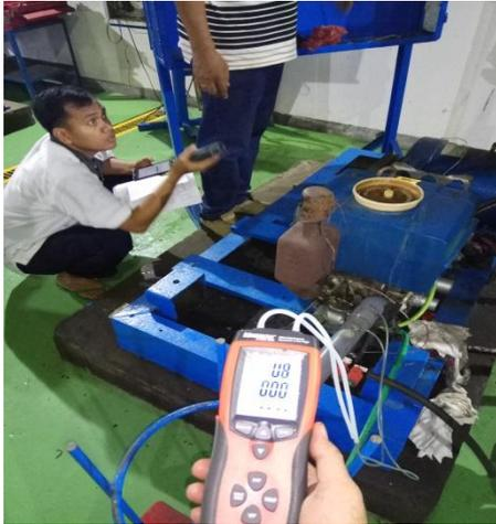
Gambar 1. Pengambilan data Mass Flow rate
