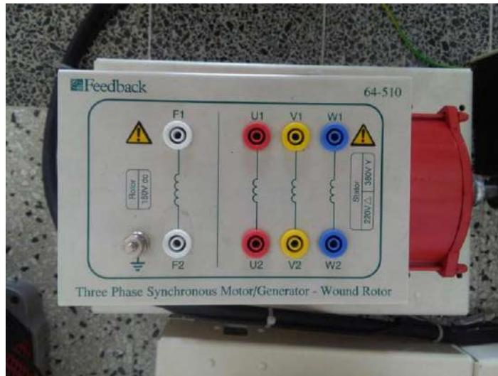
Gambar 3. 4 *Three Phase Synchronous Motor/Generator - Wound Rotor*
