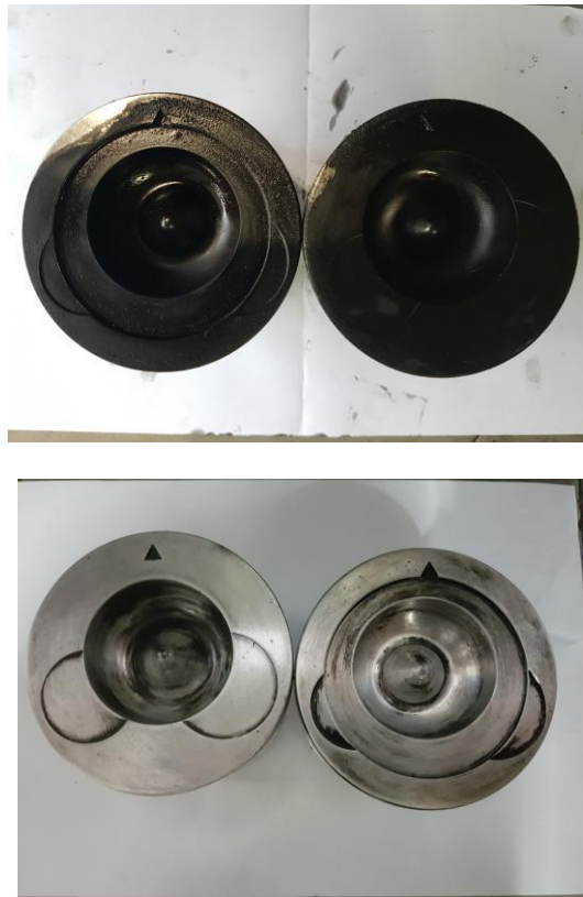
Figure 4.15. Modification piston from CR 1:18 to CR 1:16
